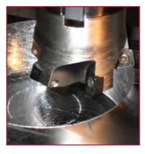
added advantage of allowing many different hole sizes to be generated with the same diameter tool. Hole size variation is all in the programming.
