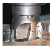
tends to avoid the high horsepower consumption characteristic of large diameter hole making. The quick and easy process offers the added advantage of allowing many different hole sizes to be generated with the same diameter tool. Hole size variation is all in the programming.
