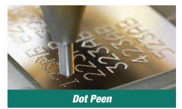
Heavy-duty dot peen marking systems in bench-top, integrated, hand-held and combo portable/bench configurations.
