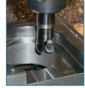
ramp angles during helical interpolation can be aggressive, without concern for rubbing the bottom of the cutting edge. This quick and easy process offers the added advantage of allowing many different hole sizes to be generated with the same diameter tool. Hole size variation is all in the programming.
